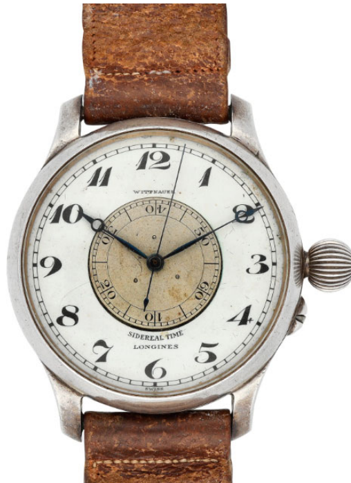
Personal Longines Weems Watch of Amy Johnson, manufactured in February 1937. Silver case of 47mm, cal. 18.69N, rotating center dial to synchronize the watch to a radio time signal. Her watch was regulated on sidereal time (marked on the dial); it served as pure navigational instrument.
